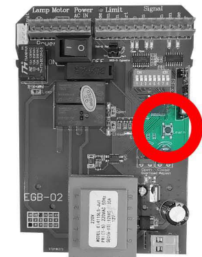
Altech EGB-02 Control Board - LEARN button (encircled by red circle)
