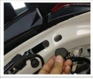
10. Remove the original rubber stopper (same left and right)
