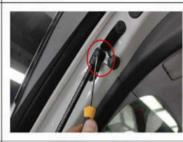
6. .Pry the gas spring snap ring and remove the original car gas spring (Same left and right)
