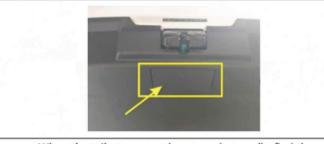
When the tailgate cannot be opened normally, find the original car emergency safety lock in the trunk, open the emergency cover and pull the emergency switch to open.
