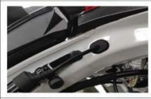
11. Thread our pole wire into the reserved hole and plug the rubber (same left and right)
