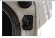
4. Remove the original car body bracket (same left and right)
