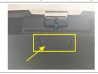
When the tailgate cannot be opened normally, find the original car emergency safety lock in the trunk, open the emergency cover and pull the emergency switch to open.
