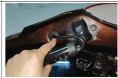
12. Insert our pole into the hole and plug the rubber plug (same left and right)
