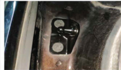
9. Use our screws to install our body bracket ("L" left "R" right)
