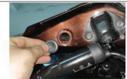
11. Remove the rubber plug reserved for the original car (same left and right)
