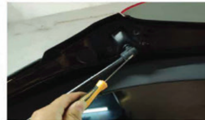
7. Pry off the gas spring snap ring and remove the left and right pole
