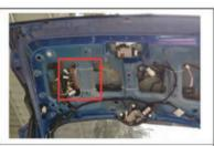
26. Connect the corresponding harness control box and fix the control box
