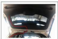
19. Pass the wiring harness of the connection control box into the corrugated pipe
