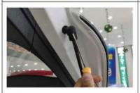
5. Pry open the gas spring snap ring, and remove the left and right side poles
