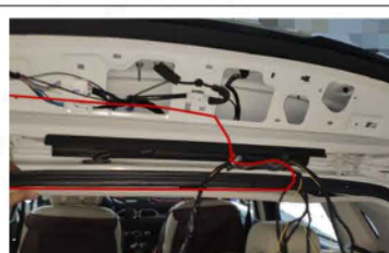
26. Thread the control box harness into the bellows
