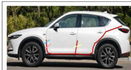
25. Threading diagram (blue: power cord, pink: front button line, yellow: unlock signal line)
