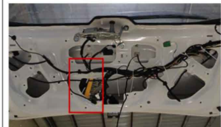
27. Connect the control box harness and fix the control box
