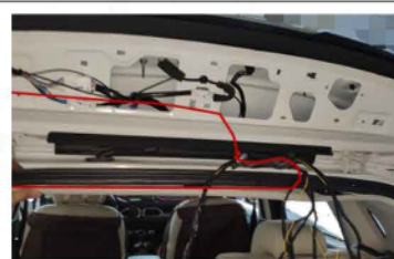
26. Thread the control box harness into the bellows
