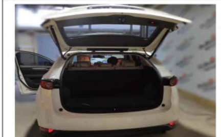
29. Recover all trims, and close the door once after installation, so as to initialize the system
