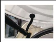
13. Thread our struts wire into the reserved hole and plug it with a rubber
