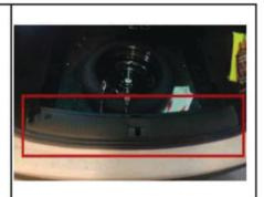
9. Remove the original car rubber(left and right are the same)
