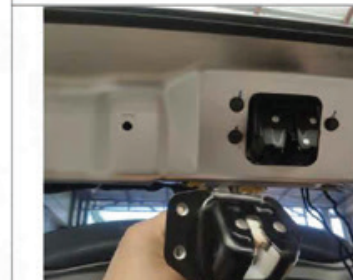
11. Remove the original car lock, Install our electric suction lock.
