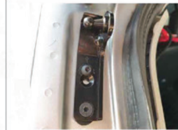
7. Install our bracket ("L" is left , " R " is right)Use our equipped screws.
