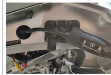
10. Put the strut wire into the hole, Plug the rubber plugs (the same left and right).
