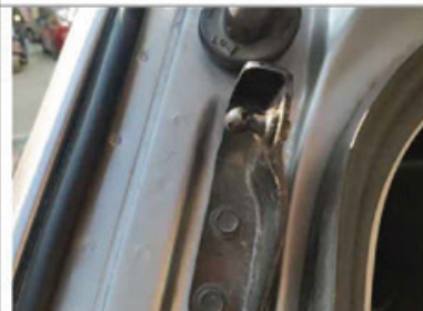
6. Remove the original car bracket (Same left and right).
