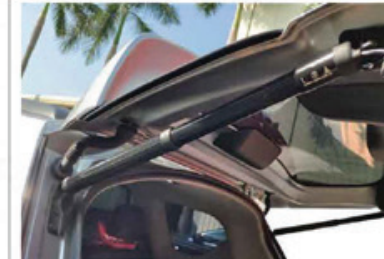
8. Install our electric pole ("L" is left, " r " is right).
