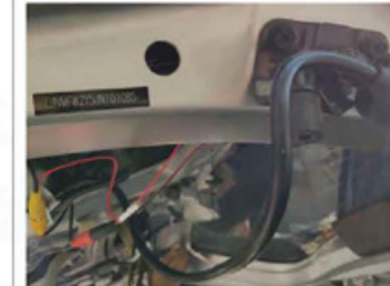
9. Make holes in the iron plate(16mm for drill).
