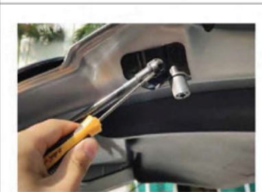
5. Use a tool to pry open the gas spring circlip, And remove the original car brace (same left and right).
