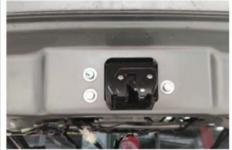
16. Remove the original lock, then install our electric upper suction lock.
