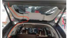
26. Routing the wire. Pass the wire harness through the fellows.
