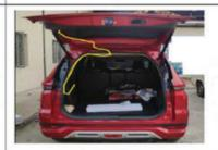
24. Pass the controller wire through rubber pipe, connect the wire to the controller.
