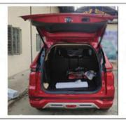
26. Installation restore , slowly manually close the tail gate once the first time for system initialization. Please cover all the decorate panels to make sure the weight the same as normal using.
