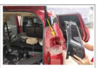
8. Pass through the electric pole's wire from taillight position.
