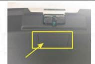
When the tailgate cannot be opened normally, find the original car emergency safety lock in the trunk, open the emergency cover and pull the emergency switch to open.
