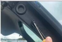
5.Use tools to pry open the original car gas spring clamp and remove the original car strut (left and right phase The same as)
