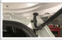
9.Thread our pole line into the reserved hole Medium, and plug the rubber plug (left and right are the same)
