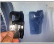
6.Remove the body support of the original car and install our body support (left of "L" and right of "R") using the screws of the original car
