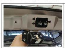
13. Remove the original lock head and install our electric suction lock head
