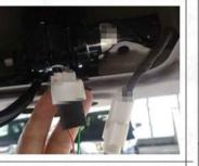
14.Unplug the original car lock plug, and our wiring harness **Relative connection**
