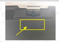
When the tailgate cannot be opened normally, find the original car emergency safety lock in the trunk, open the emergency cover and pull the emergency switch to open.
