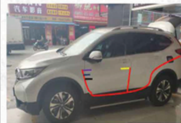
21. Threading diagram (purple: power wire, black: front button wire, yellow: unlock signal wire)
