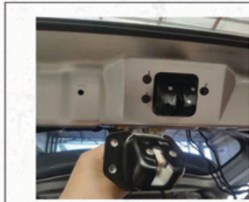
13. Remove the original car lock and install our upper suction lock
