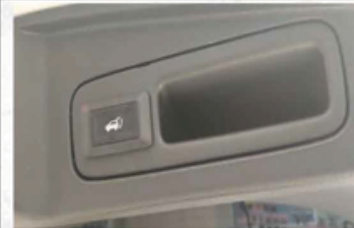
23. Remove the original car pull box and install our special tail door button
