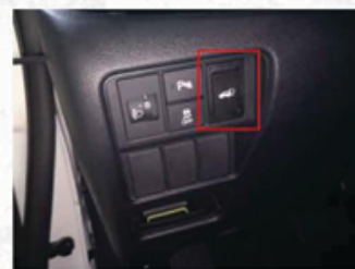
18. Remove the reserved button of the original car and install our dedicated front button
