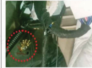
20. The power ground wire is on the left side of the trunk
