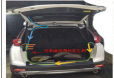
22. Blue: control box wiring harness, yellow: strut wire, orange: negative power line
