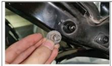
7. Remove the original rear door screw ball and install our screw ball
