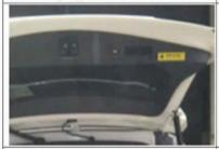
23. Punch holes in the trim panel of the tail door to install the rear switch
