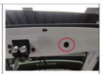
20. Punch holes in the appropriate position of the tailgate to install the tailgate buttons
