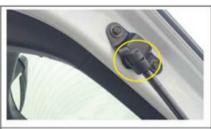
7. Pry off the gas spring retainer and remove the original vehicle gas lever
