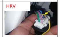
15. Our yellow line is connected to the original car unlock signal line (XRV: original purple line)
