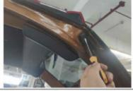
4. Pry open the gas spring snap ring and remove the original car strut (same left and right)
