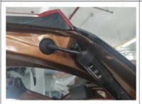
9. Thread our pole wire into the punched hole and plug the rubber plug (same left and right)
