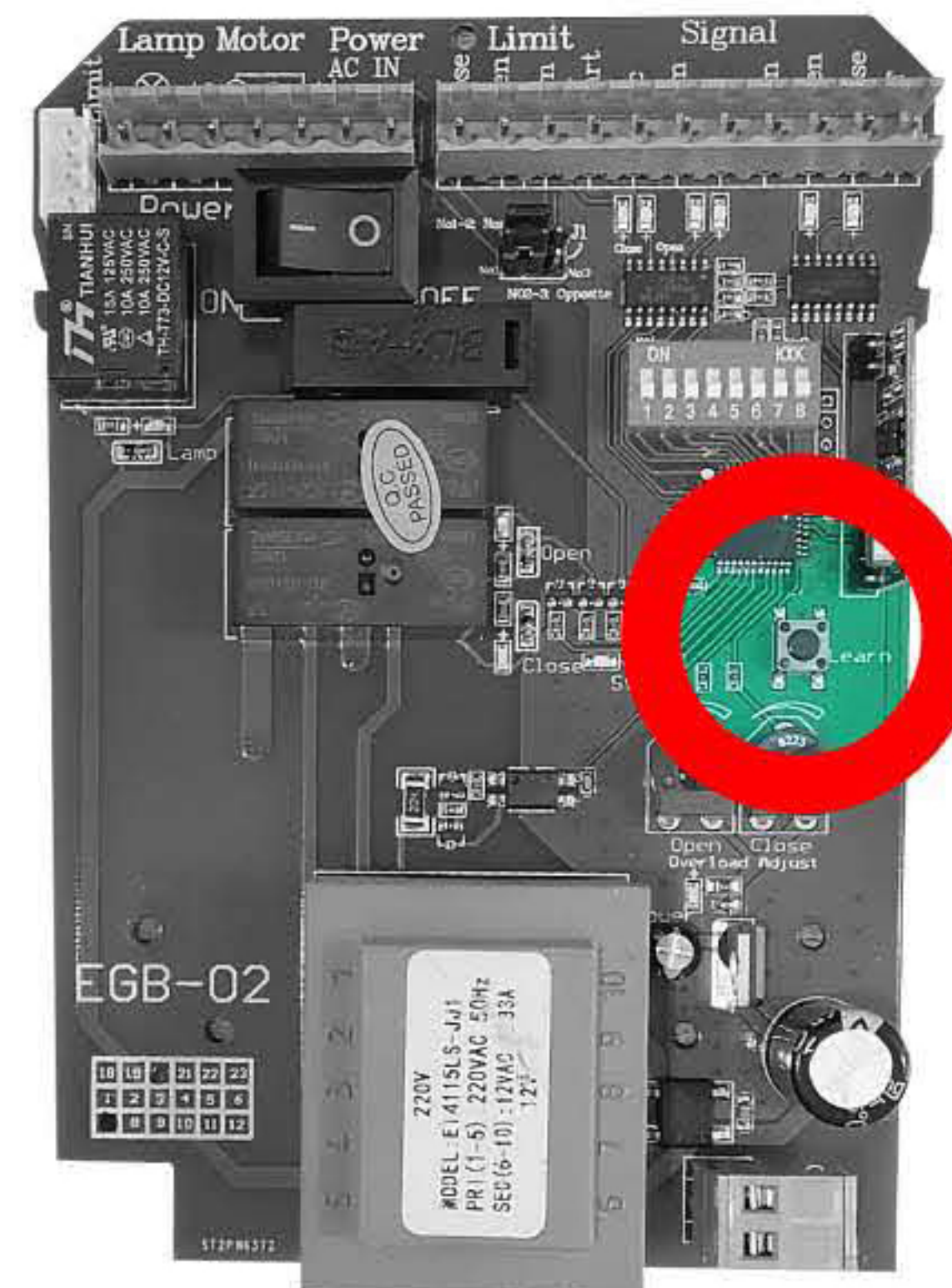
Altech EGB-02 Control Board - LEARN button (encircled by red circle)
