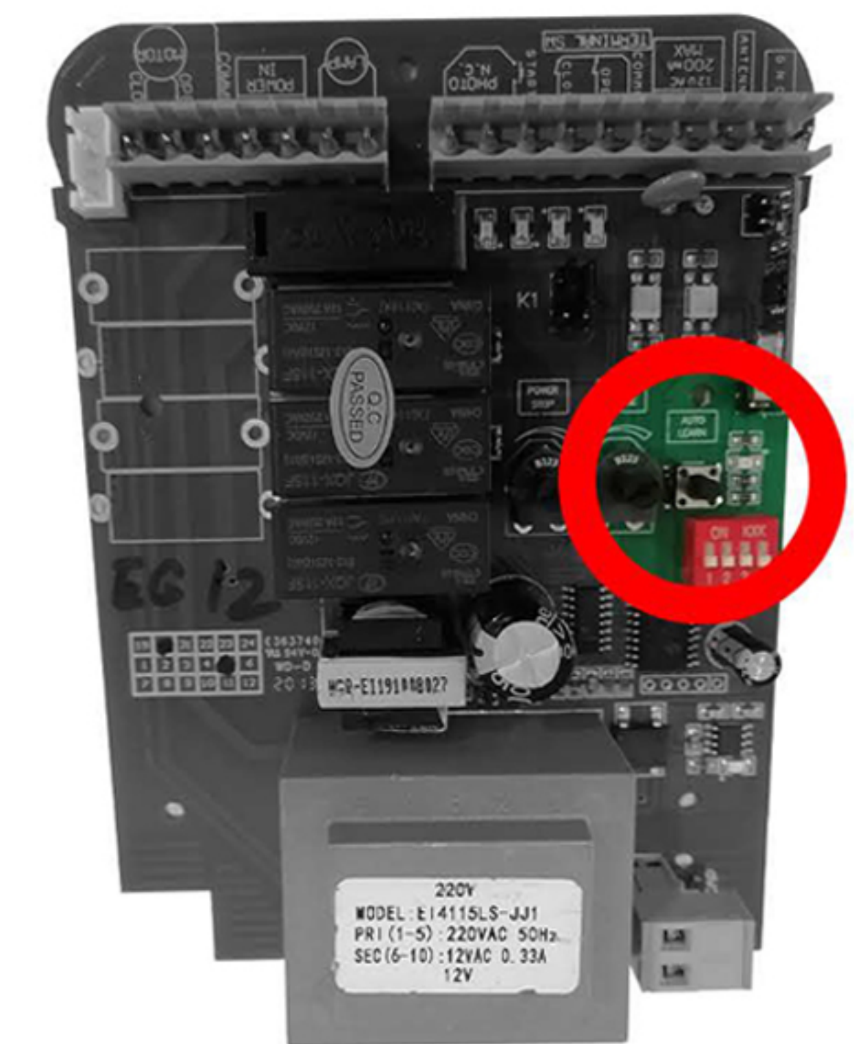
Altech EG-12 Control Board - LEARN button (encircled by red circle)
