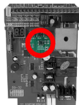
Altech EG-32 Control Board - LEARN button (encircled by red circle)
