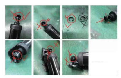
Qualified ball head circlip
