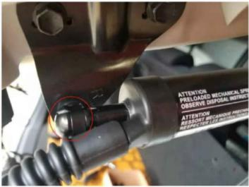
Remove the lower support of the original vehicle, replace it with our company's support, and install our company's support rod (the same installation method for both sides)
