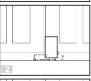
2. Fix the lock body onto the first moving side of the gate leaf, make sure there is at least 5 to 8 mm space between the stopper location hole surface & the bottom of lock body.
